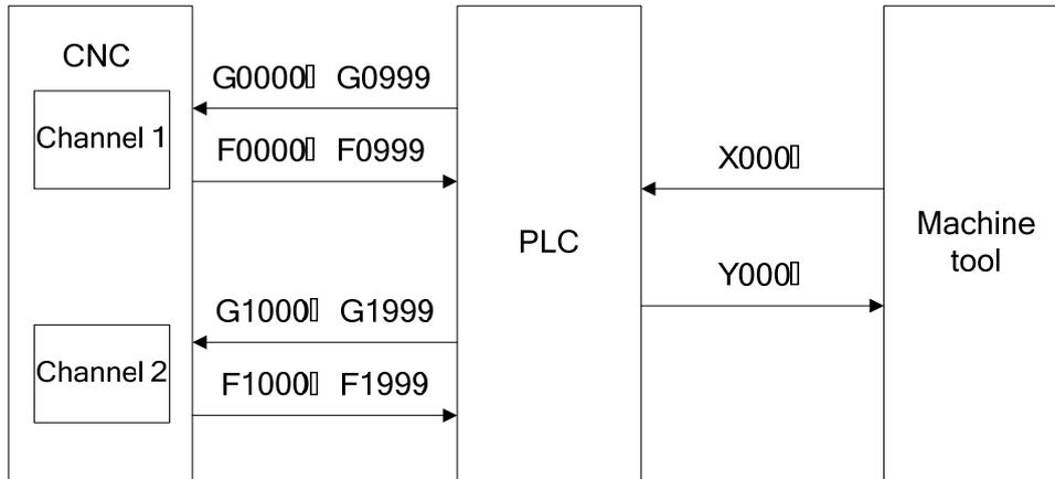
In the following address expressions, “n” means that the used address position of each channel at the CNC side.
