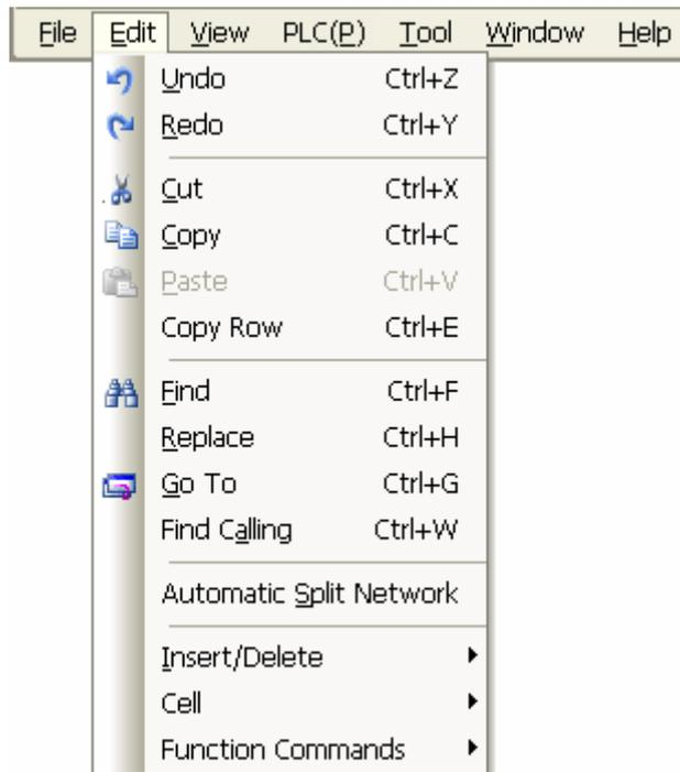
It should be noted that the last three items in “Edit” menu “Insert/Delete”, “Cell” and “Function Commands” are only displayed in the Ladder View.
