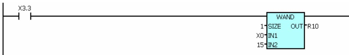
Explanation: When X0003.3=1, ANDs the data (8 digits) in X0 and 15 (binary: 00001111), the result is stored in R10. For example, when X0003.0=1, and X0=11000110, after the WAND instruction is executed, the result in R10 is 00000110.
