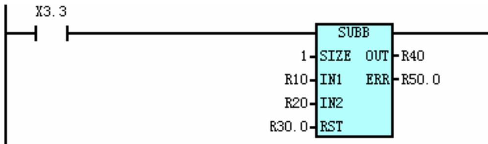
Explanation: When X0003.3=1, SUBB instruction is executed, R0040=R0010-R0020; If the calculation is erroneous, then the R0050.0 is 1, otherwise R0050.0 is 0. When R0030.0 is 1, the state of R0040 remains the same and R0050.0 is reset to 0.
