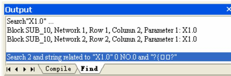
In Ladder View, the type of parameters (constant, addresses or symbols) can be exclusively searched according to the input character string. The options such as “Exact Match” and “Match Case” are available only when the symbols or function commands are searched. “Match Case” is invalid when searching for addresses. Both “Exact Match” and “Match Case” are invalid when searching for constants. For address, formats “x0.1” and “X0000.1” represent the same one and will lead to the same result.
