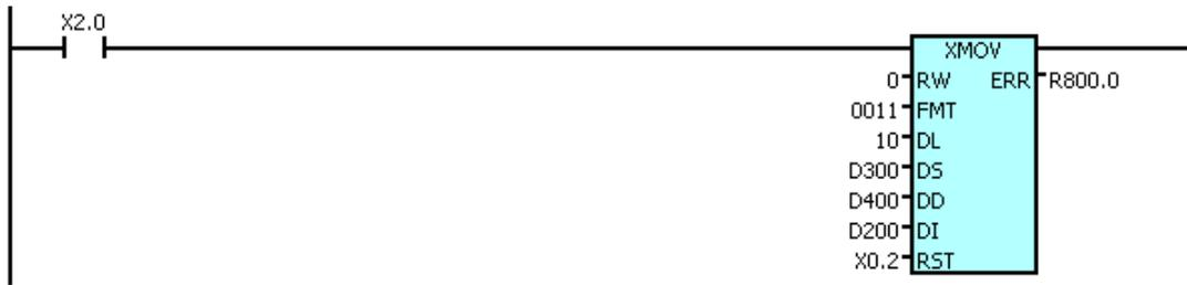
Explanation: It is supposed to D200=3, D303=500, PLC offsets the data value in D200 by the initial address D300 of the resource data when X2.0 sets to 1; the address after offset is regarded as D303. Then, transmit the data from D303 to the destination address D400, that is, D400=D303=500; if the command execution is error, R800.0 sets to 1; the R888.0 is cleared when X0.2 sets to 1.
