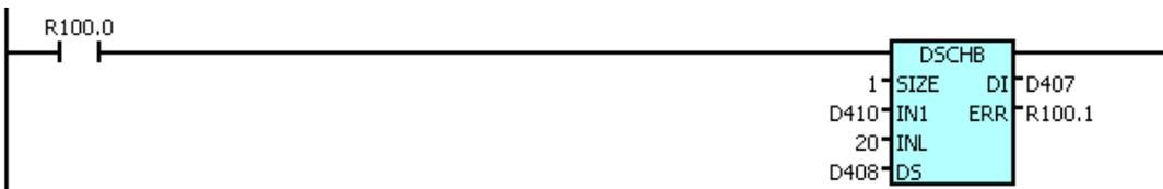
Explanation: When R100.0=1, index whether the same data within the D408 are existed inside the D410-D429, for example: when the data D408 in the D420 is identical, the D407 output data is 10. If this range does not include the same data within the D408, output ERR, R100.1=1, D407 data resets to 0.
