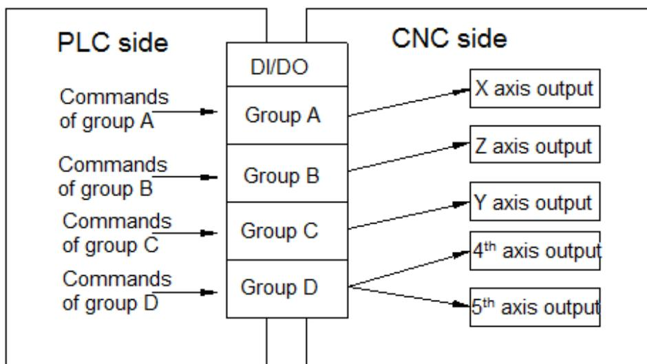
**Note 1: The relation between the group and the axis is set by the data parameters (select DI/DO group for each axis controlled by PLC);**
