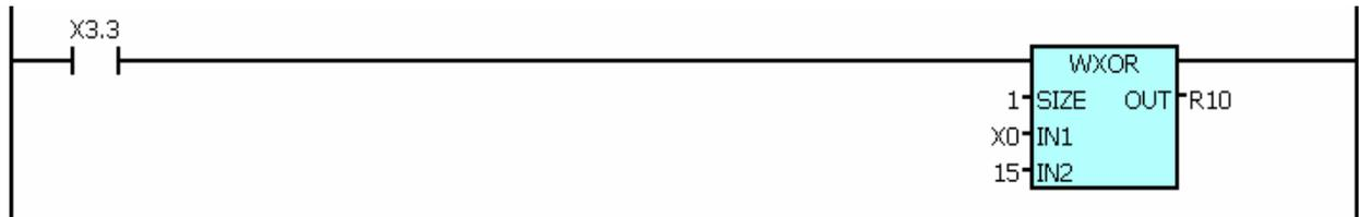
Explanation: When X0003.3=1, XORs the data in X0 (8 digits) and 15 (binary: 00001111), the result is stored in R10. For example, when X0003.3=1 and X0 = 11000110, after the WXOR instruction is executed, the result in R10 is 00001001.
