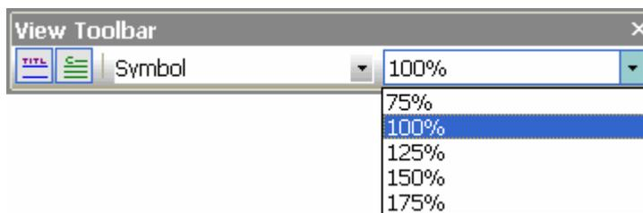
The scaling ratio can be 75%, 100%, 125%, 150% or 175%. They can be set via the on Ladder View Toolbar.
