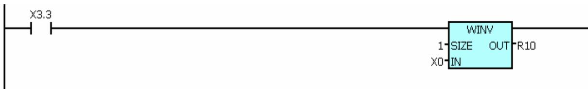
Explanation: When X0003.3=1, inverses the data (8 bits) in X0 and stores the result in R10. For example, when X0003.3=1 and X0=11000110, after the WINV instruction is executed, the result in R10 is 00111001.
