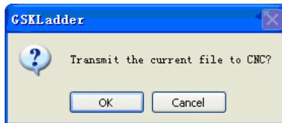
The setting of CNC user level should be more than 2 levels when the file is being transmitted, otherwise, the prompt “CNC authority prohibits to modify the file data” occurs.
