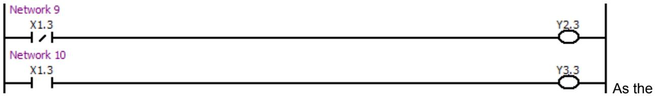
As the above-mentioned shows, at the beginning, if the X1.3=0, X1.3 immediately turns into 1 after Y2.3=1, in this case, perform the next ladder diagram, so that Y3.3=1; the Y2.3 and Y3.3 will be simultaneously regarded as 1. In order to avoid this occurrence, the short pulse signal can be treated with synchronization; refer to the following figure:
