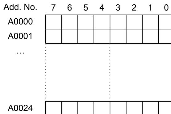
When editing the ladder diagram, each address A corresponding to an alarm number; Whether the corresponding address A is PLC alarm or PLC alert can be performed by setting the alarm numbers within different range. Alarm types from the alarm number are slightly different based upon the different system types.
