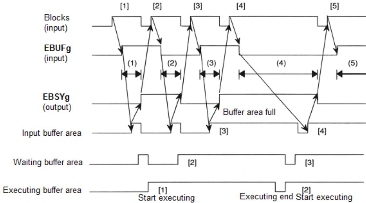
(1), (2), (3), (4), (5), during the interval, the new block can't be sent (i.e. When EBUFg and EBSYg are in the different logic status, the new block can't be read in).
