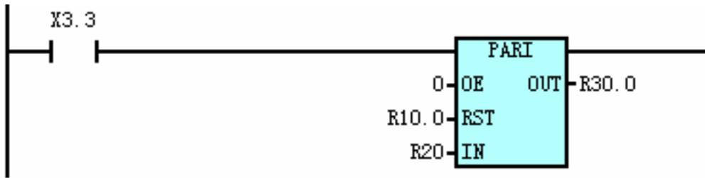
Explanation: If PARI is executed when X0003.3=1, OE=0000, parity check is performed. When R0010.0=1, R0030.0 is reset to 0, parity check is not performed. When R0010.0=0, parity check is performed. R0030.0 is 0 when R0020 data contains even parity; R0030.0 is 1 when R0020 data contains odd parity.
