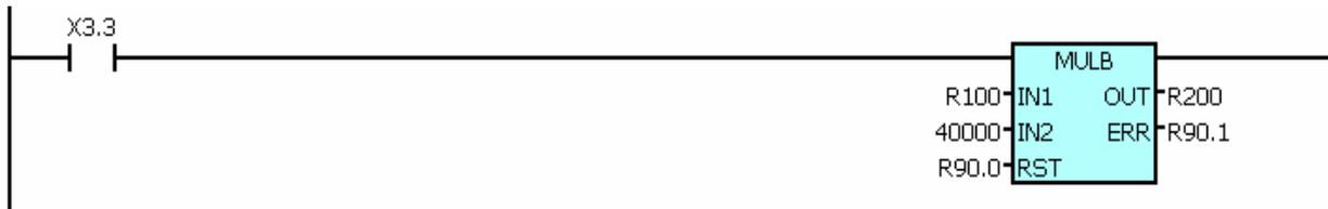
Explanation: When X0003.3=1, the data consisting R100 and R101 (16 bits, R101 takes up high 8 bits, R100 takes up low 8 bits) is multiplied by constant 40000, and the product is stored in the 4 bytes whose start address is R200 (R200, R201, R202, R203, R200 takes up low 8 bits).
