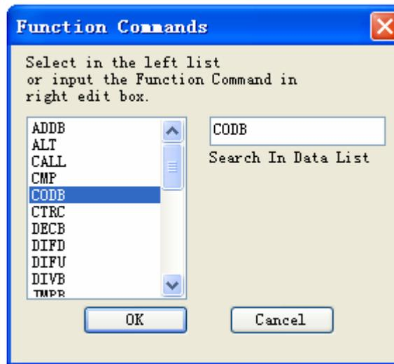
The function commands are selectable in the left side and can also be entered in the edit box. Double-click the command or click [OK] after entering the command. The execution result is the same as executing the commands in submenus.
