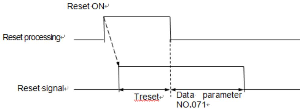
During the Auto operation, the automatic operation is stopped when CNC is reset; the machine tool decelerates and then stops along with the movement direction of the controllable axis. When the CNC is reset during executing the M, S and T commands, the MF, SF and TF signals within 16ms are set to “0”.
