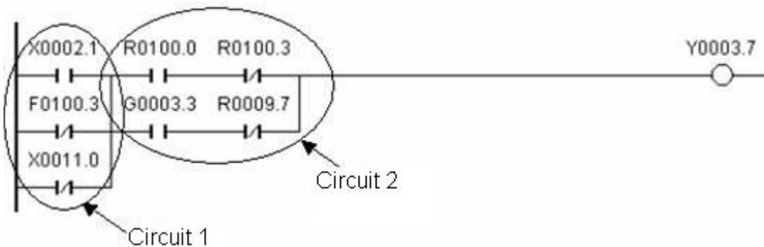
Explanation: ORB indicates the serial circuits in parallel in circuit 2; ANB indicates the circuit 1 and circuit 2 are connected in series.
