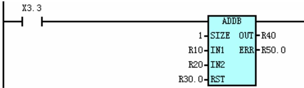
Explanation: When X0003.3=1, ADDB instruction is executed.  $R0040=R0010+R0020$ ; If the operation is erroneous,  $R00500.0=1$ , otherwise  $R00500.0=0$ ; When  $R0030.0=1$ , the state of  $R0040$  remains unchanged, and  $R0050.0$  is reset to 0.
