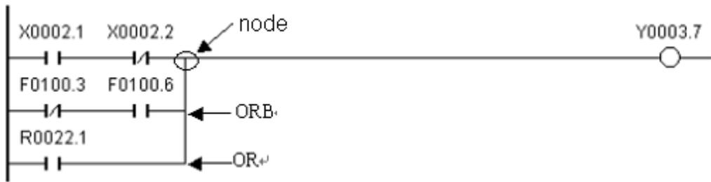
Explanation: There are three branches (0002, 0003, and 0004) from the left bus to the node. Branches 0002 and 0003 are serial circuits. When there are serial circuits connected in parallel between the bus to the node or node to node, ORB instruction is used for the all the branch ends except for the first branch. As branch 0004 is not serial circuit, OR instruction can be used.
