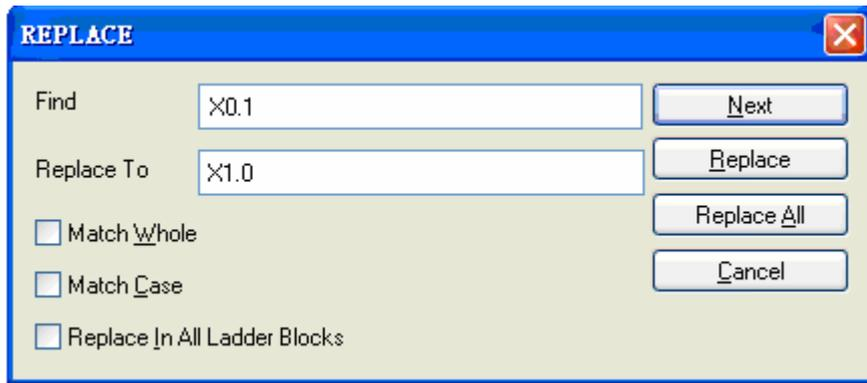
The find function in REPLACE dialogue box is the same as in [Find]. Replacement can be executed only when the search condition is fulfilled and the input content is legal. Address (or bit address) cannot be used to replace constant (or byte address), and vice versa.
