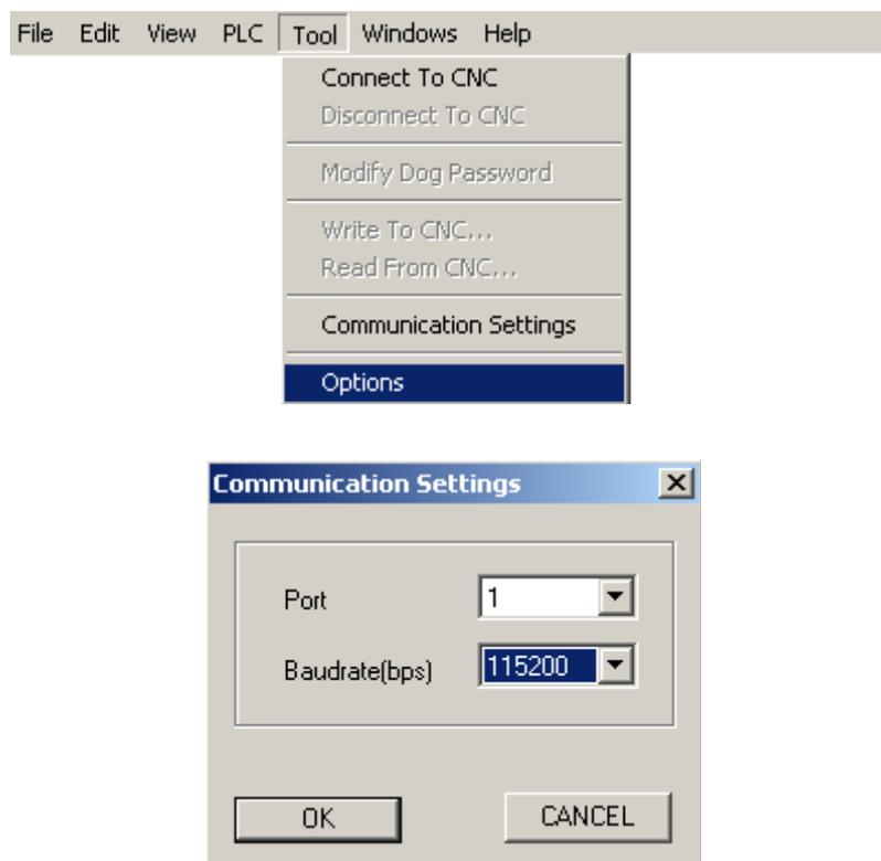
GSKLadder adopts the method that the communication is immediately transited while connecting. Namely, it is disconnected between GSKLadder and CNC when the transmission does not perform. It is only connected based upon the demand of transmission; the connection can be automatically cut off after the transmission is completed. Therefore, it is enough to perform the “transmit to CNC” or “transmit from CNC” when transmitting.
