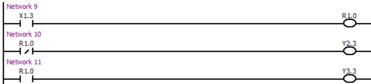
After the synchronization treatment is performed, when X1.3=1, the Y3.3=1 and the Y2.3=0; when X1.3=0, Y2.3=1, Y3.3=0, therefore, the occurrence of which the Y3.3 and Y2.3 are shared with 1 will not happen.
