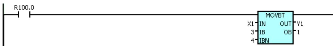
Explanation: When R100.0=0, the state of Y1 is invariable; when R100.0=1, the 4<sup>th</sup> digit of the 3<sup>rd</sup> bit of the X1 transmits to the start position at the 1<sup>st</sup> digit of Y1, that is, Y1.1=X1.3, Y1.2=X1.4, Y1.3=X1.5 and Y1.4=X1.6.
