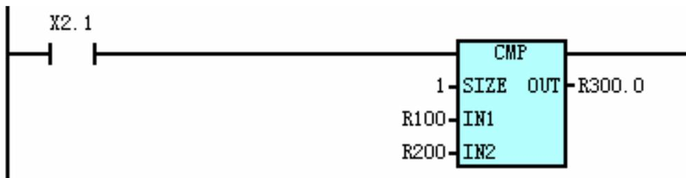
Explanation: When X0002.1 is 0, the comparison is not performed; the states of R0300.0, R0300.1 and R0300.2 remain unchanged.
