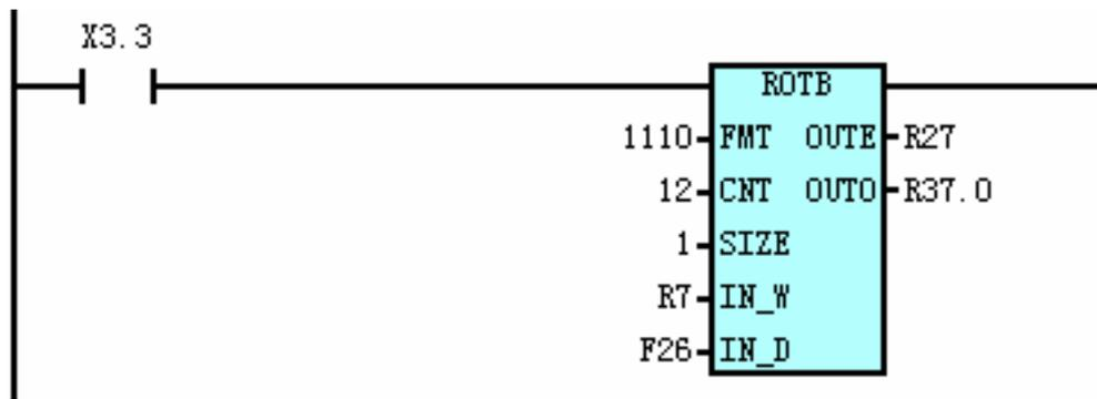
When the short path rotation is performed, the position number of the previous position before the object position is calculated. The current position number  $R0007=1$ , rotary table indexing position number  $CNT=12$ , then when  $X0003.3=1$ :
