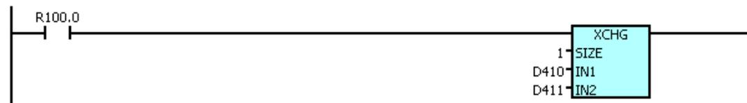
Explanation: When R100.0=0, the data in the D410 and D411 are invariable; when R100.0=1, the data in the D410 and D411 are exchanged; that is, write the data from D410 to the D411; write the data from D411 to D410.
