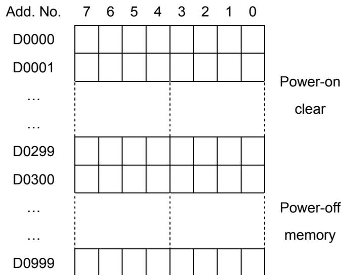
The D address of GSK980TD<sub>c</sub>, GSK980MD<sub>c</sub> or GSK980TTC is 4-byte and its data length is 32-bit.
