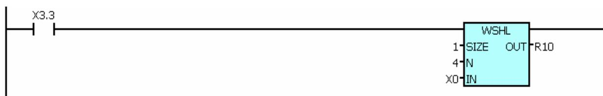
Explanation: When X0003.3=1, it shifts left 4 bits of the data (8 bits) in X0, and the result is stored in R10. For example, when X0003.3=1, and X0=11000110, after the WSHL instruction is executed, the result in R10 is 01100000.
