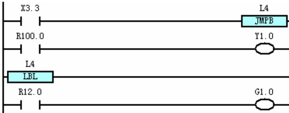
Explanation: When X0003.3 is 1, the program jump over R100.0 and executed from R12.1; if X0003.3 is 0, the execution starts from R100.0.
