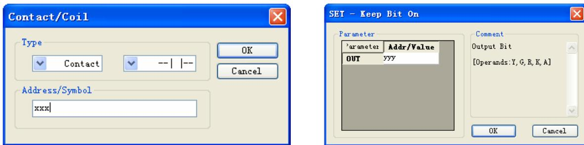
When a parameter is displayed in “Address” view, the symbols which represent the parameter are displayed in blue; if the symbols are invalid or undefined, they are displayed in red. In “Symbol” view or “Address: Symbol” view, symbols are black when the parameter is correct; when the mapping address type is not the required one, the symbol is orange; symbols are red when they are incorrect or undefined.
