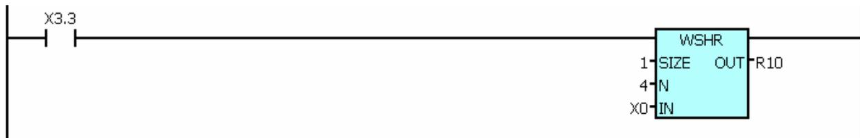
Explanation: When X0003.3=1, it shifts right 4 bits of the data (8 bits) in X0, and the result is stored in R10. For example, when X0003.3=1, and X0=11000110, after the WSHL instruction is executed, the result in R10 is 01100000.
