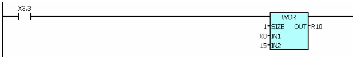
Explanation: When X0003.3=1, ORs the data in X0 (8 digits) and 15 (binary: 00001111), and stores the result in R10. For example, when X0003.3=1 and X0 is 11000110, after the WOR instruction is executed, the result in R10 is 00001111.
