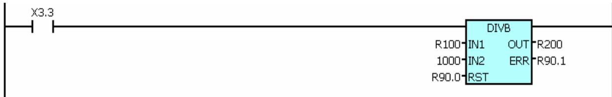
Explanation: When X0003.3=1, it divides the data (16 bits, R101 takes up high 8 bits, R100 takes up low 8 bits) consisted of R100, R101 and constant 1000, and the result is stored in the 4 bytes whose start address is R200 (R200, R201, R202, R203, R200 takes up low 8 bits), the remainder (16 bits) is stored in two bytes (R202, R203, R202 takes up low 8 bits) whose start address is R202.
